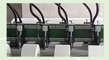
Both Pneumatic cutter or Electrical cutter can be customized on machine, user can according production request to choose the suitable cutter for machine.
