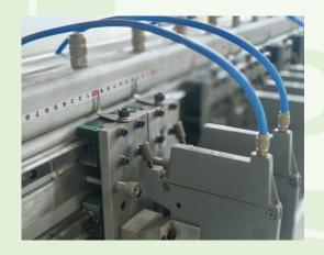
By adjusting the position of the blade, user can easily control the cutting width.
