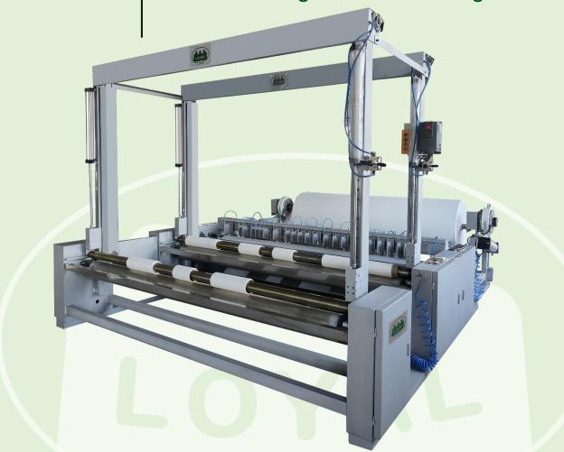
Fully automatic slitting and re-winding machine, working from original gauze rolls (from loom or after bleaching process).
