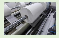
Specially designed to obtain pre-cutted gauze rolls to be used in the feeding of our automatic gauze swab folding machine (SERIE SS-ZDG) for the production of swabs (compresses).
