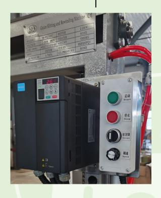
Frequency converter controls the speed, make constant tension and linear velocity, precise speed regulating, stable running, and accurate counting.
