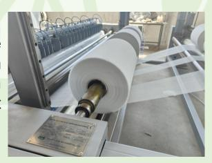
During winding, the tension control device works to make it suitable to cut raw gauze with too many joints and unbalanced tension.
