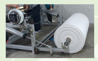
The raw material holder has regulating function which can adjust the position of gauze jumbo roll position within range of +2.5cm.
