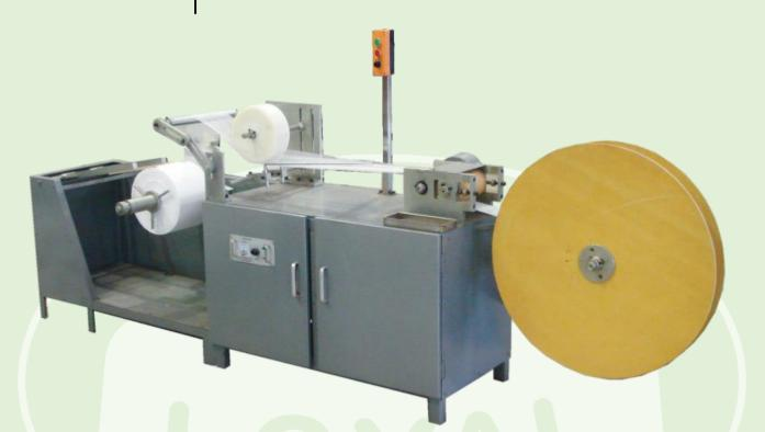
Series single wheel folding and rewinding machine folds the gauze lengthwise into several plies and rewinds for the preparation of swabs.
