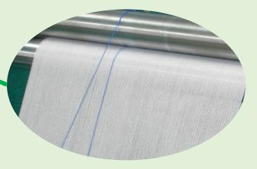
On-line perm X-RAY detectable thread function can be customized.
