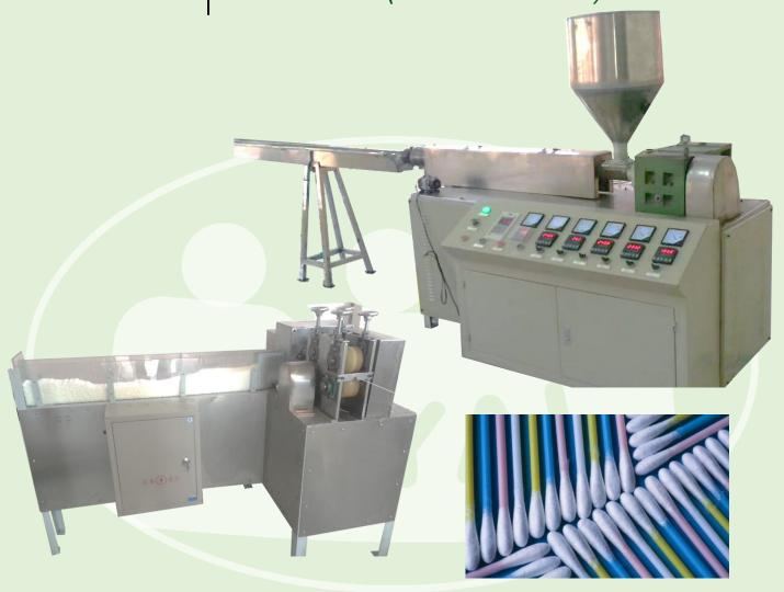
Automatically making the plastic stick (use for produce cotton swabs), machine composed of plastic extruder, cooling system, cutting and output systems.
