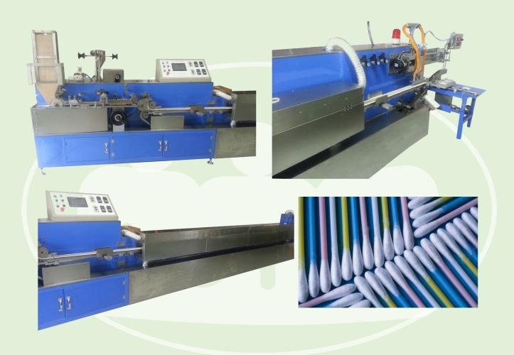
Automatically making and packing cotton swabs with PLC program control system, closed-air drying system, defective products remove and replenish system and vacuum suction packing system.
