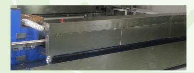
Double hot air closed drying system save power and control the cotton buds dryness at 5%.
