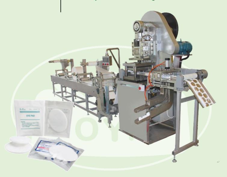
Machine do automatic combine multi layers of material, punching and making output with counting function.
