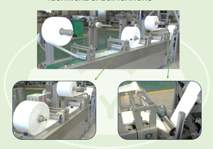
The material unwinding by conveyor, avoid cotton roll been fracture.
