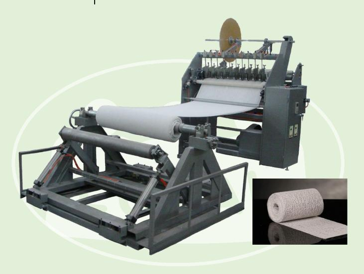
Automatically unwinding, deviation correction, slitting, length counting, re-winding, auxiliary demount.
