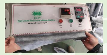
Via change parts of the machine, user can easily make shoe cover size change length from 40-45cm (accept customized).
