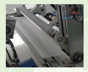
Winding system winding the gauze material at pre-set length, automatically make cross cutting and output to the paper wrapping process.
