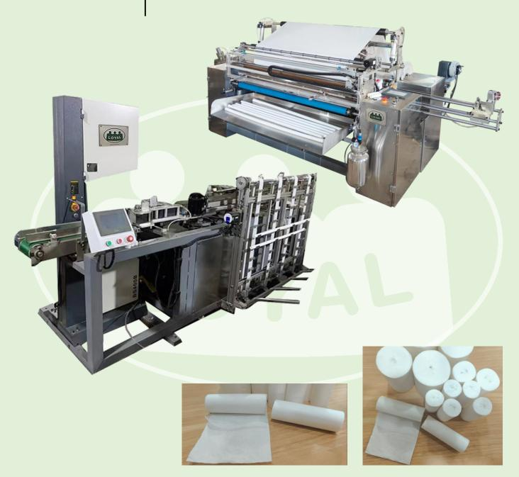
Automatically make bandage winding, wrapping with paper and cutting.
