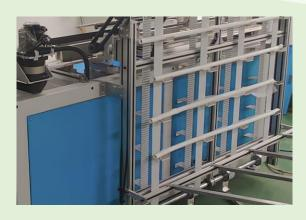
After winding and wrapping paper process, the bandage roll been transferred to the cutting system through the lifting mechanism.
