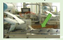
For smaller size product packing, machine can do customize as 3 lanes, it will increased the production capacity 1.5 times.
