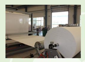
The automatic tension control system responses sensitively, responds fast, be qualified for different gram weight of spunlace non-woven fabric, maximum guarantee spunlace (very sensitive tension) non-woven not been deformation during the slitting and rewinding process.
