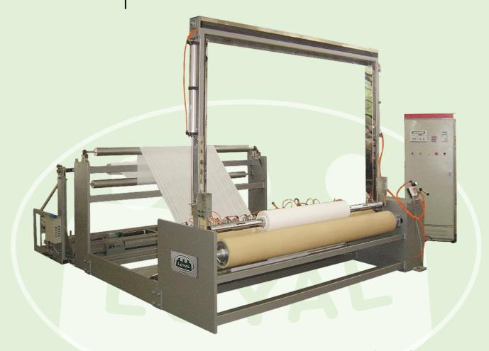
It is suitable for slitting and rewinding 20~120g/m2 Spunlace non-woven jumbo roll material.
