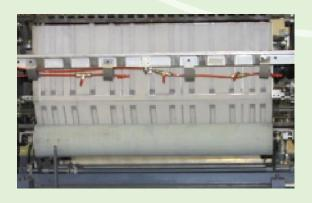
Key part--cuter, it is made by alloy tool steel, available to use in a long service life.
