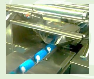
A special designed forming box can be quickly adjusted to fit different size of products.
