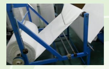
Production process start from raw material cotton roll feeding, then conveying to embossing, cutting, counting, output.
