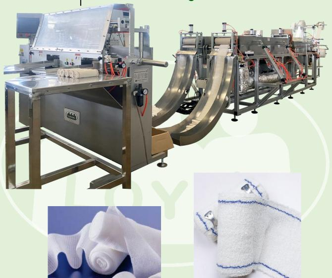
The production line is composed of humidifying system, hot air drying system and bandage coreless winding system, suitable for make many types of elastic bandage.
