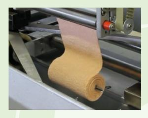
Cutting at pre-set length with a pair of specially-designed scissors, it makes cutting accurate and clean. After cutting, the materials will automatically feed in.
