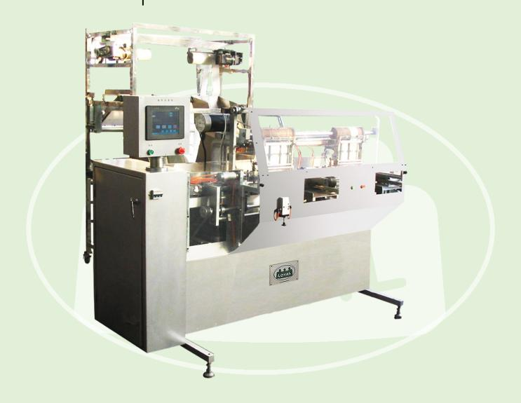
Automatically unwinding the materials rolls, feeding, winding, length counting, cutting and output the bandage.
